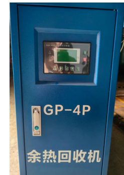
Waste Heat Recovery Machine
