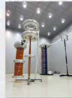
3,000kV impulse voltage generator and 1,000kV power frequency withstand voltage and partial discharge test system
