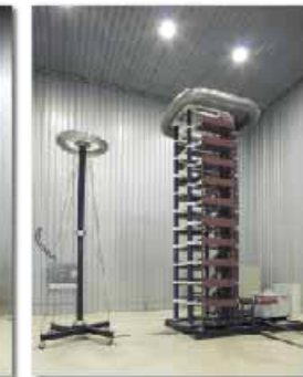
Test transformer, coupling capacitor and impulse voltage lead-in bushing and 1,500kV impulse voltage generator
