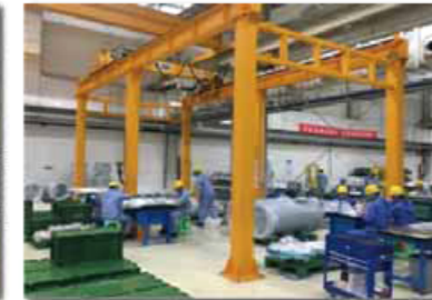
Sub-assembly Workshop 100,000 Cleaning Grade, covers an area of 5,000m 2
